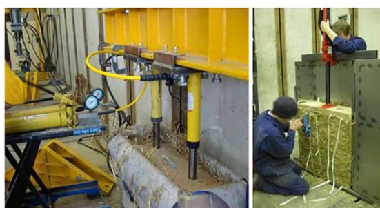
Figure 3 Equipment used to create test bales at the University of Bath.
