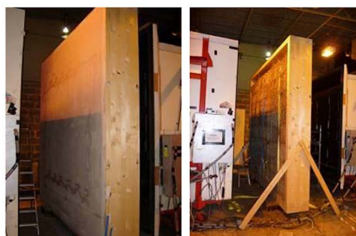
Figure 5 Prefabricated ModCell panel and Guarded Hot Box facility at the BBA, Garston, UK.
