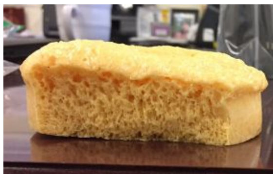
Figure 8. NIPU foam produced by carbonated linseed oil
