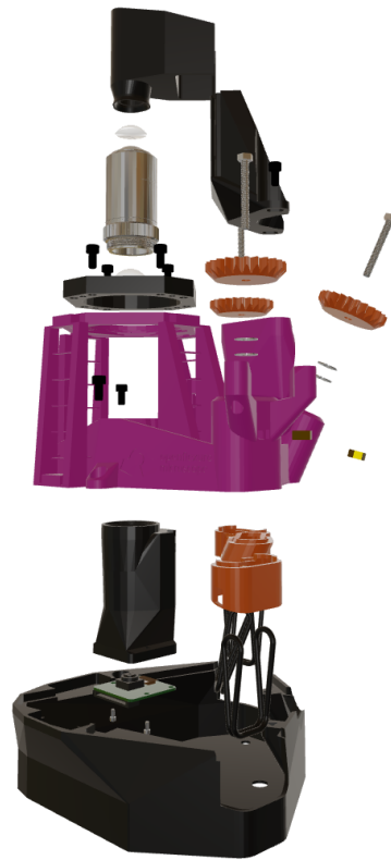
Fig. 1. Exploded view of the OpenFlexure Microscope.
