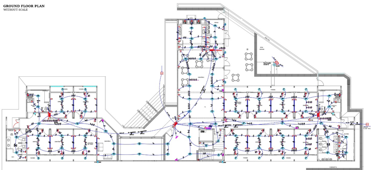
Figure 4: Ground Floor Electric Plant of Original Design in dwg Format (Source: USP São Carlos Campus City Hall, 2019).
