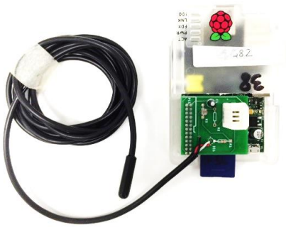
Figure 3 - The temperature, relative humidity, and a Passive Infrared Sensor (PIR) used in this study
