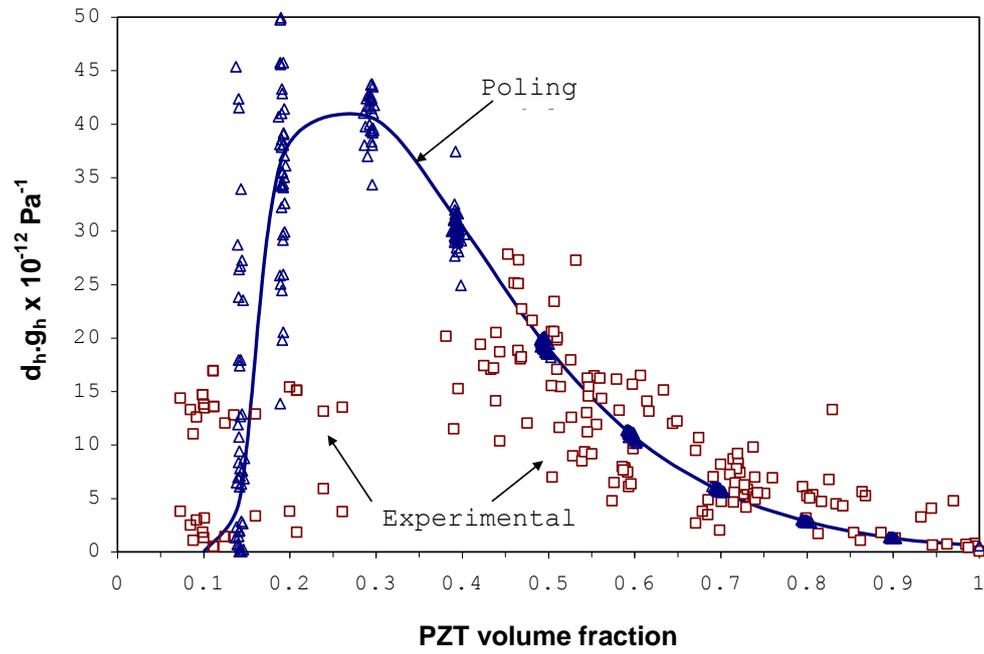
Figure 8. Variation of  $d_h \cdot g_h$  as a function of PZT volume fraction. Experimental data from
