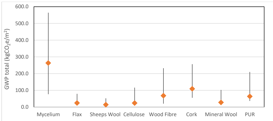
Figure 4 A to C Total GWP range. In orange the UK base scenario GWP. The black line represents the maximum and minimum GWP obtained in all the scenarios investigated.
