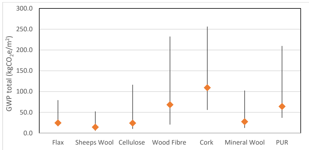
Figure 5 A to C Total GWP range excluded mycelium. In orange the UK base scenario GWP. The black line represents the maximum and minimum GWP obtained in all the scenarios investigated.
