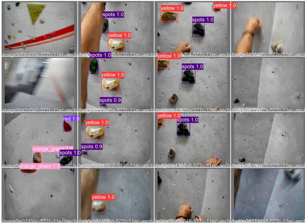
Figure 2: A sample batch of validation images and predictions created by YOLOv5 during the hold detection training process. Each batch contained 16 images, each with a resolution of 320 × 240 pixels.
