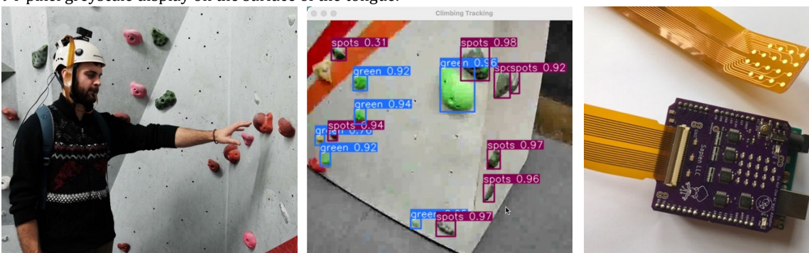
Figure 1: Climb-o-Vision in use (left). Climbing hold identification visual render (center). The Cthulhu Shield tongue interface output device (right).
