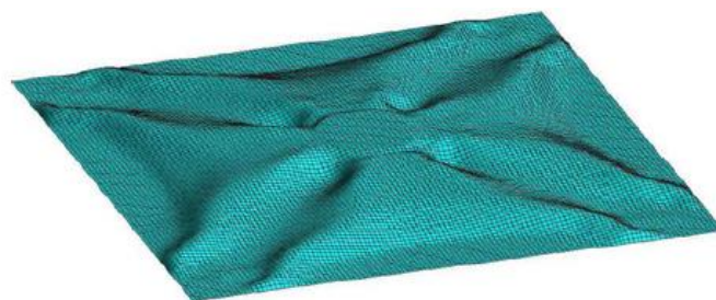
699 (b) Shape optimisation of a sheet subject to out-of-plane loads (reprinting permission for 700 these images has been obtained from the publisher [158]).
