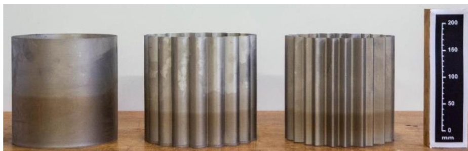
693 694 (a) Reference stainless steel circular shell and optimized, Aster and wavy shells 3D 695 printed by powder bed fusion (reprinting permission for these images has been 696 obtained from the publisher [157]). 697
