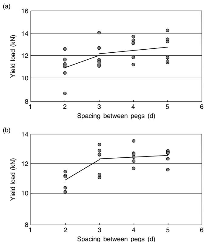
**Figure 6.** (a) Spacing between pegs versus yield strength of connections with  $a_{3t}$  of 2d; (b) Spacing between pegs versus yield strength of connections with  $a_{3t}$  of 3d
