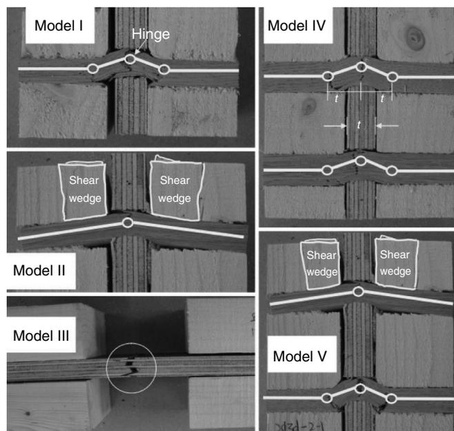
Figure 3. Failure modes observed from the tests
