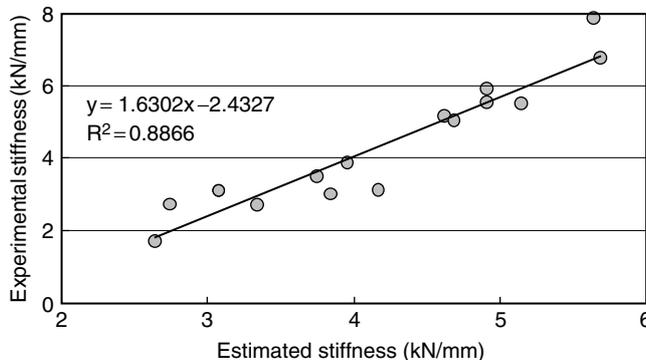
**Figure 9.** Comparison of estimated and experimental stiffness
