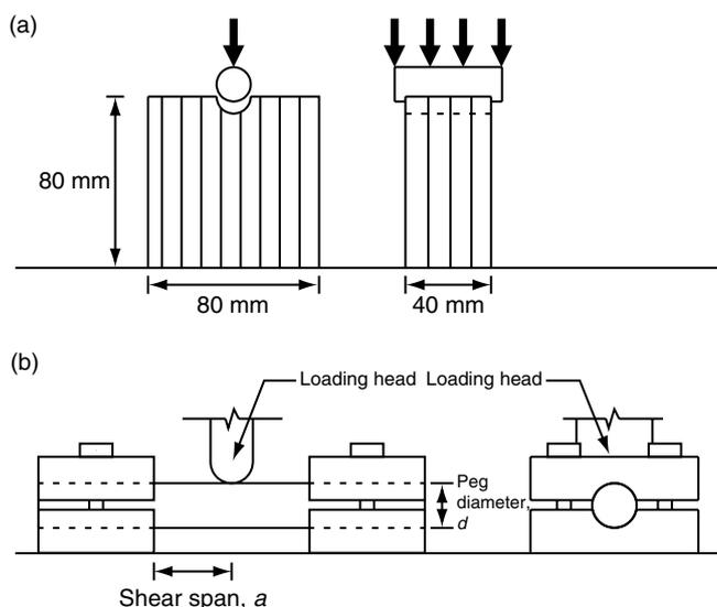
**Figure 1.** (a) Test apparatus for bearing strength test; (b) Test apparatus for fixed-fixed ends bending test
