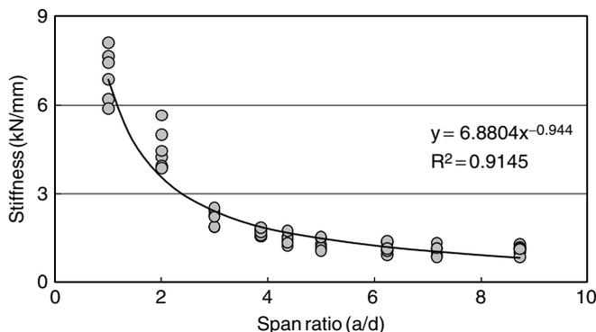
**Figure 8.** Shear span ratio versus stiffness of pegs
