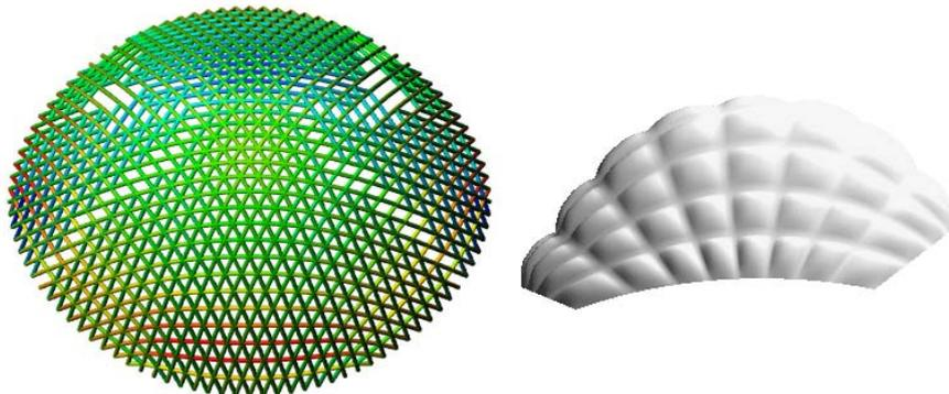
*Fig. 5 Optimisation results, removing unstressed members (left) and ETFE formfinding (right)*
