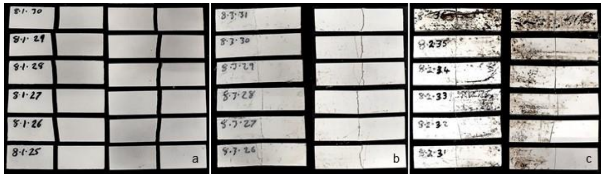
Figure 6 - Flexural test specimens subjected to the two-year fungal treatment showing the extent to which fungal growth can be observed on the exterior of the fibrous plaster, and the variation in extent within samples. a) NF2 – no treatment, no fungal growth evident. b) BF2 – subjected to fungal treatment, some growth evident. c) AF2 – subjected to fungal treatment and shows very significant fungal presence on the sample specimens.
