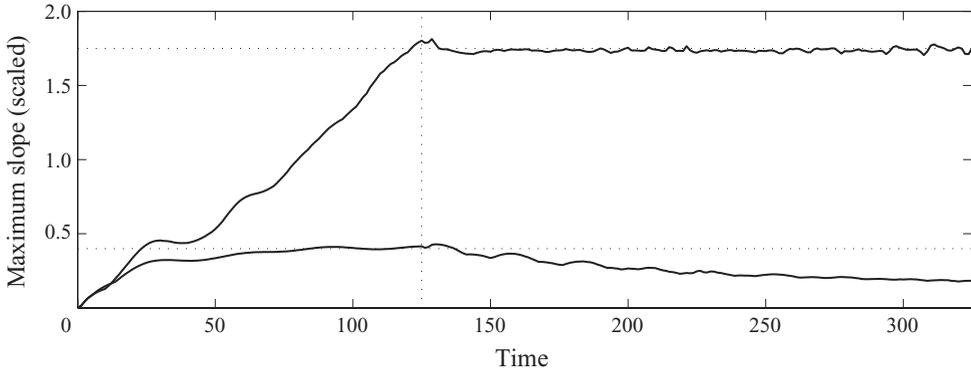
FIGURE 5. Maximum slope of the free surface as a function of time for the computations shown in figures 3 and 4. The forcing was turned off at  $t = 125$ . The lower curve has been vertically magnified by a factor of 10 to reflect the difference in forcing amplitude.
