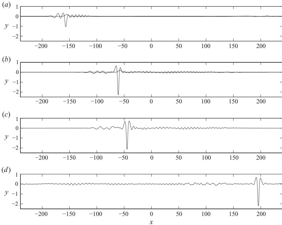
FIGURE 4. Time-dependent computation of the free surface due to a subcritically moving force at larger forcing amplitudes ( $a=0.2$ ,  $s=1.3$ ). The forcing was switched on at  $t=0$ ,  $x=-220$  and switched off at  $t=125$ . The solution, together with the forcing, is shown in (a–d) at times  $t=50$ , 125, 137.5, 325, respectively. The forcing is also shown.
