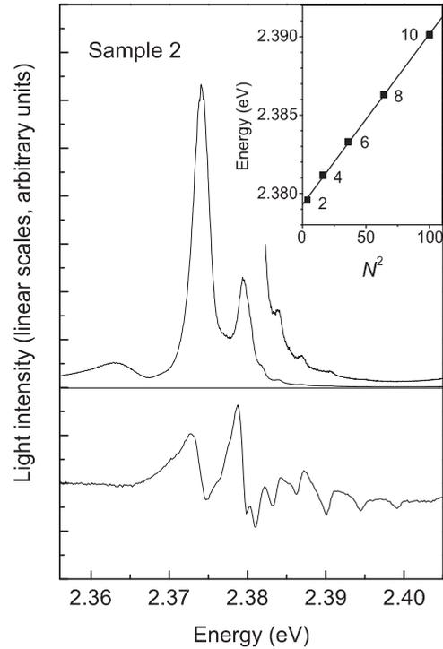
FIG. 1. Reflectivity (lower panel) and photoluminescence (upper panel) spectra from sample 2 ( $L = 80$  nm,  $S = -6$  meV) at 1.6 K in zero magnetic field. The inset shows the c.m. transition energies plotted against the square of the translational quantum number  $N$ , whose values are indicated in the diagram. For this value of  $L$  and for  $N > 1$ , the signals for even values of  $N$  are much stronger than those for odd values (see, e.g., Refs. 6 and 7).
