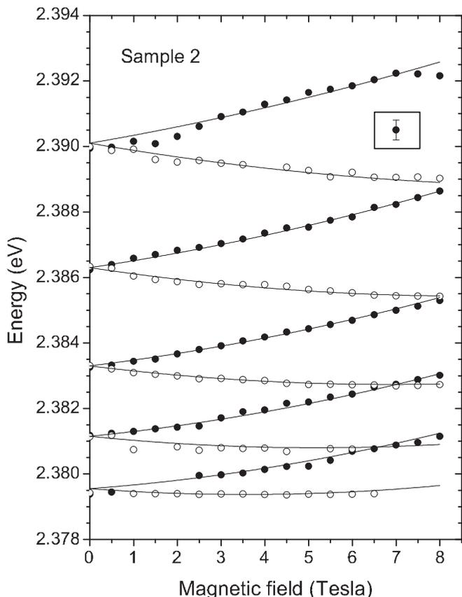
FIG. 2. The dependence of the transition energies of sample 2 as a function of magnetic field at 6.8 K. Filled and open symbols are for  $\sigma_+$  and  $\sigma_-$  transitions, respectively. The continuous lines are of the form given by Eq. (1). The error bar indicated in the inset corresponds to the full width at half maximum of a typical signal.
