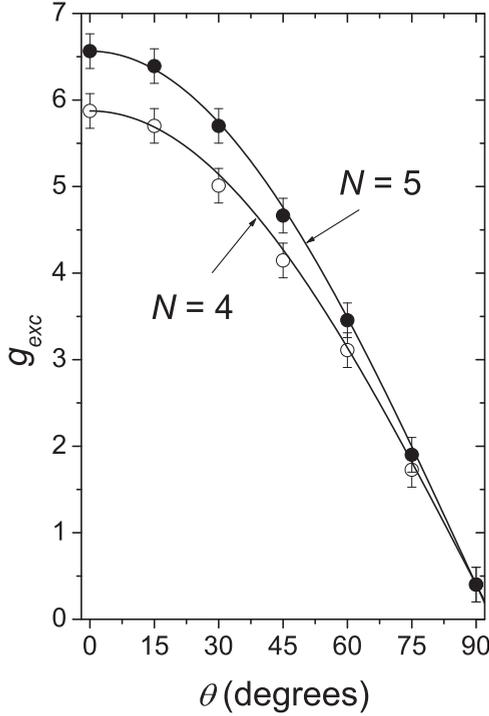
FIG. 4. Dependence of the exciton  $g$  value on the angle  $\theta$  between the magnetic field and the growth axis for the  $N = 4$  and  $N = 5$  transitions in sample 1 ( $L = 100$  nm,  $S = -5$  meV). The curves are of the form given in Eq. (2).
