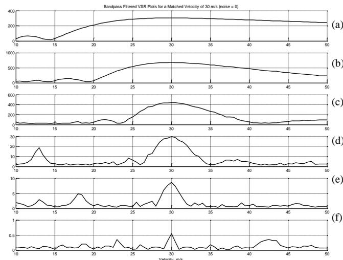
Figure 4. Bandpass filtered version of the IVS plot shown in Fig 2 using TMAP function #1 to generate an SFAP with a propagation velocity of 30 m/s. The filters are 8<sup>th</sup> order Butterworth digital units with centre frequencies  $f_0$  are (a) 1 kHz, (b) 2 kHz, (c) 4 kHz, (d) 8 kHz, (e) 16 kHz and (f) 32 kHz. The corresponding values of  $Q_v$  are 1.4, 2.9, 5.7. The velocity step is 1 m/s and there is no additive noise.
