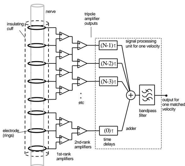
Figure 1. This shows a *multi-electrode cuff (MEC)* connected to a *tripolar* (double differential) amplifier array. The  $N$  tripolar outputs (where  $N$  is typically about 10) are digitised and processed in the signal processing unit on the right of the figure.
