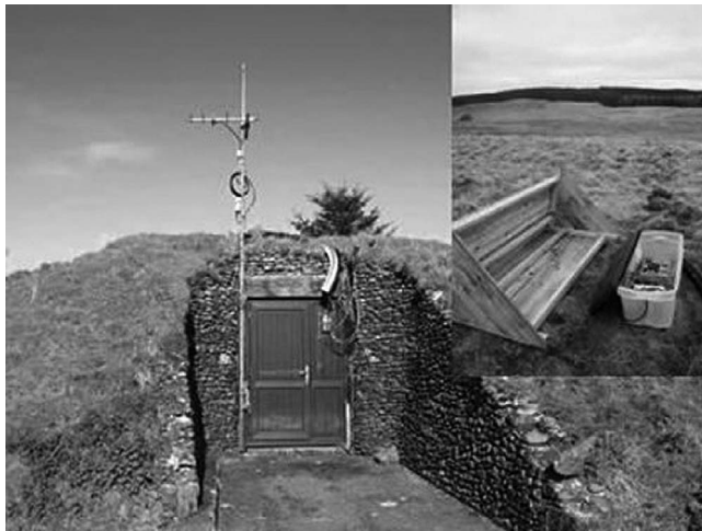
Figure 3. The seismic vault entrance at Eskdalemuir, Scotland, with the ADU and sensors behind the hill shown in the inserted photo.
