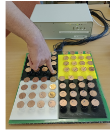
Fig 2: Photograph of 16-channel MIT instrument and 16-coil planar array with deformable membrane skin fitted, where a single membrane element of the skin is shown manually displaced or touched.
