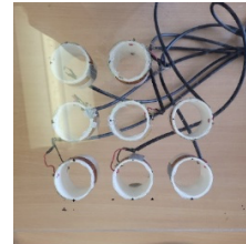
Fig. 3: The 8-coil array sensor, indicating the coil distribution.
