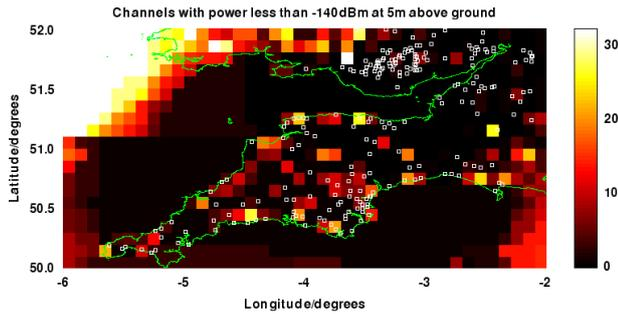
Fig. 9. Increasing the protection limit from -120 dBm (Fig. 4) to -140 dBm would make the available resource very scarce.
