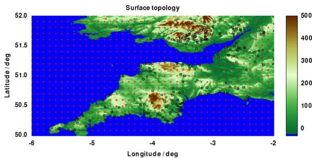
Fig. 10. The terrain height in the south-west of the UK. The crosses indicate where the spectrum occupancy was sampled. The black squares indicate the location of the transmitters.
