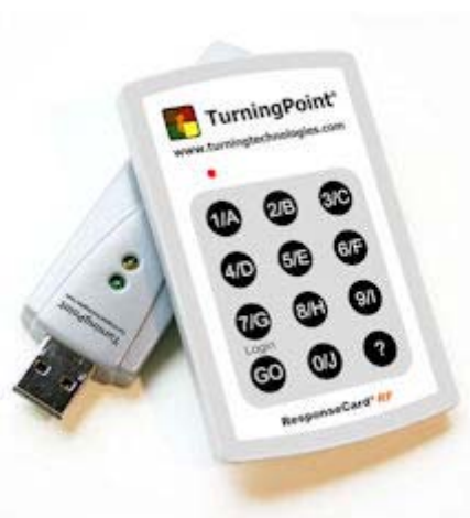
Figure 2: The EVS hardware – the USB RF receiver (left), together with a clicker.
