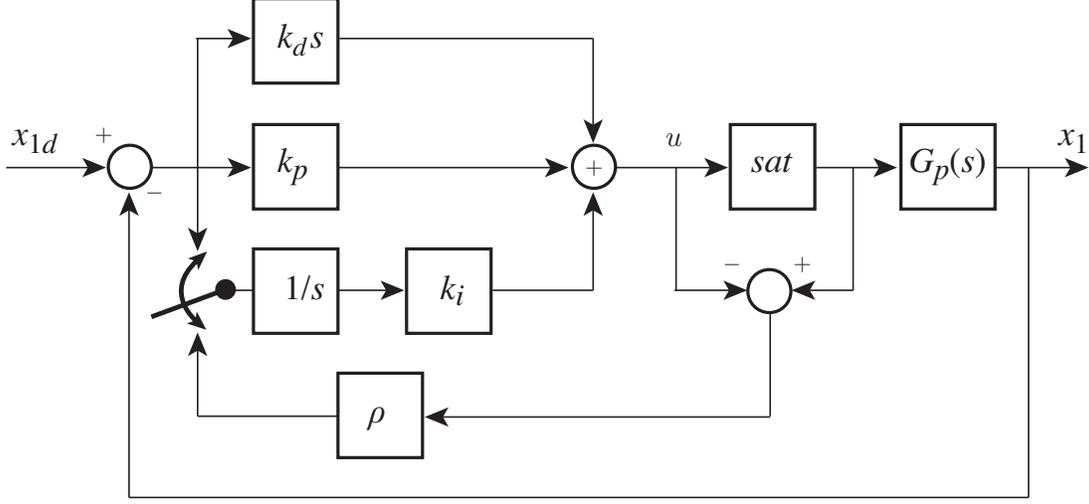
Figure 9: Block diagram of variable structure PID controller.
