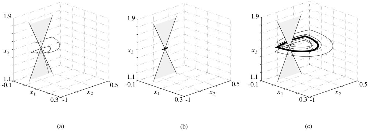
Figure 7: Orbits of the MIMO system for  $b_{31} = -0.01$  (a),  $b_{31} = 0.05$  (b), and  $b_{31} = 0.2$  (c). The upper grey triangle is the escaping region  $\Sigma^e$  and the lower grey triangle is the sliding region  $\Sigma^s$ . The crossing regions are not depicted. The thick curves in (b) and (c) are stable limit cycles.
