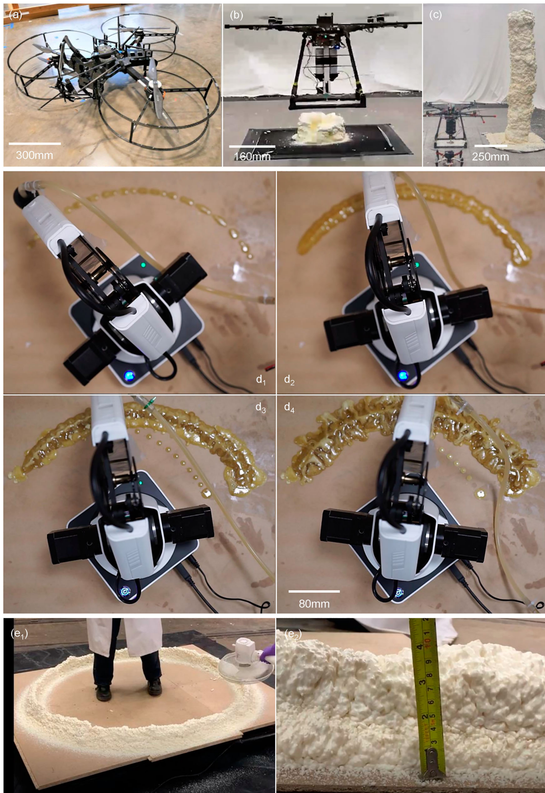
Figure 13. Autonomous deposition of freshly mixed, uncured foam material. (a) Grounded UAV suitable for Aerial-AM deposition. (b) The experimental platform: flying base and parallel UAV depositing a bead of low-density foam material in a circular trajectory showing Aerial-AM in action. (Adapted from an AAM project video sequence [50]). (c) A low-density foam extrusion 1 m tall. (d) Dobot magician robot arm depositing high-density foam in a programmed arc trajectory, shown at two ( d_1 ), four ( d_2 ), six ( d_3 ) and eight ( d_4 ) layers. (Full details of the deposition device used are contained in [48]). (e) Test print of the spray low-density foam in a circular trajectory of 1.5 m diameter with three layers and application of a fan to assess any effects of downwash (left) and two layers printed showing variation in layer height (right).
