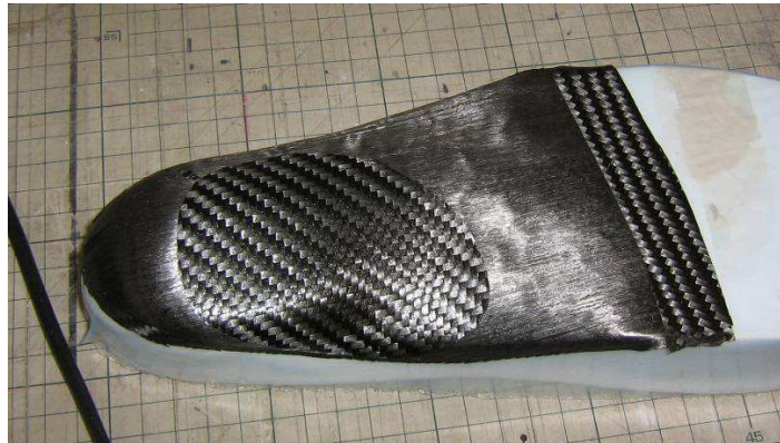
Figure 6: Laying up process
