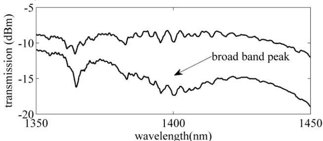
**Fig. 10. Fiber D transmission spectrum measured just after fabrication (top), and after 28 weeks of exposure (bottom). Note the surface peak growth and the appearance of a broad absorption feature.**
