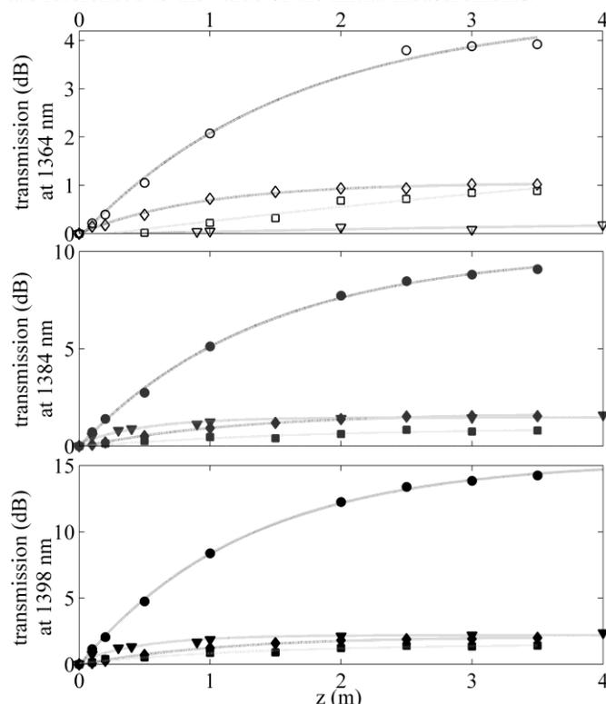
**Fig. 8. Comparison of the exponential fits and experimental normalized transmission for the localization of degradation at one of the contaminated ends. From top to bottom 1364 nm, 1384 nm and 1398 nm. Data points: circles correspond to a diameter of 1.3  $\mu\text{m}$ , diamonds to 2.5  $\mu\text{m}$ , triangles to 5.2  $\mu\text{m}$  and squares correspond to the HC-PCF.**
