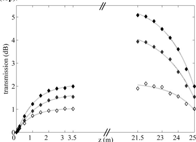
**Fig. 6. Transmission of different absorption bands for fiber B (2.5  $\mu\text{m}$  core diameter). The dotted lines correspond to the exponential fits and diamonds to data points at 1364 nm (white), 1384 nm (gray) and 1398 nm (black),  $z$  is the fiber length. The transmission increases as the contaminated ends are chopped. On the left the comparison for fiber B at one fiber end.**
