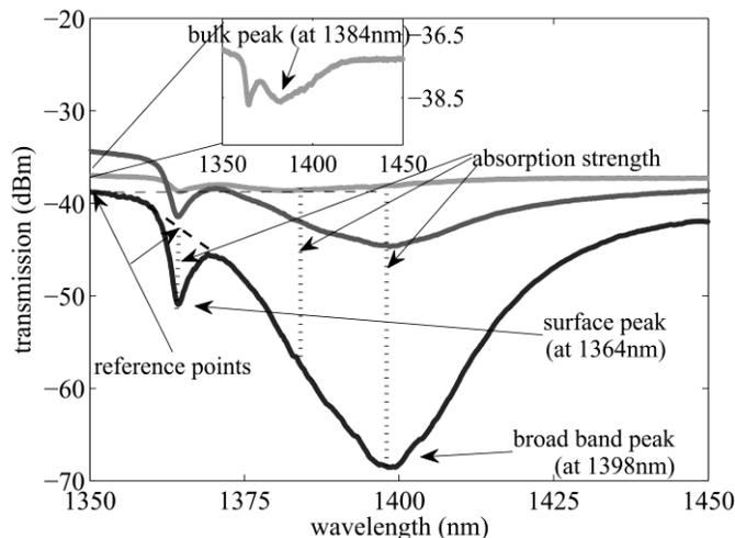
**Fig. 3. Transmission for fiber A (1.3  $\mu\text{m}$ ) for different exposure times. From light gray to dark gray the exposure time was: day 0, week, 4 and week 22 (the different signal level is due to a difference in the input coupling). Dotted lines illustrate the absorption strength (modulus of the difference between the reference points and the wavelengths 1364 nm, 1384 nm and 1398 nm). The inset is a y-axis zoom of the first measurement.**
