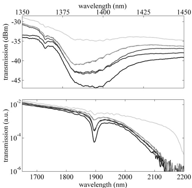
**Fig. 7. Transmission (from 1350 nm to 1450 nm and from 1650 nm 2200 nm) for a low loss 5  $\mu\text{m}$  core fiber exposed over 2 years to atmospheric conditions. Transmission measured over (in both wavelengths ranges from bottom to top) 249 m, 243 m and recoupling onto the other end 243 m, 237 m and 50 m.**
