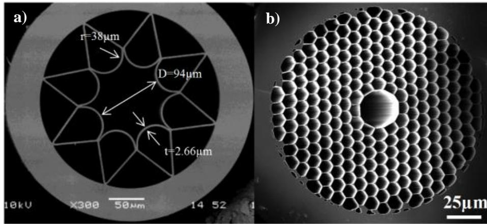
**Figure 2: SEM pictures of the hollow core fibres used for this work.**
