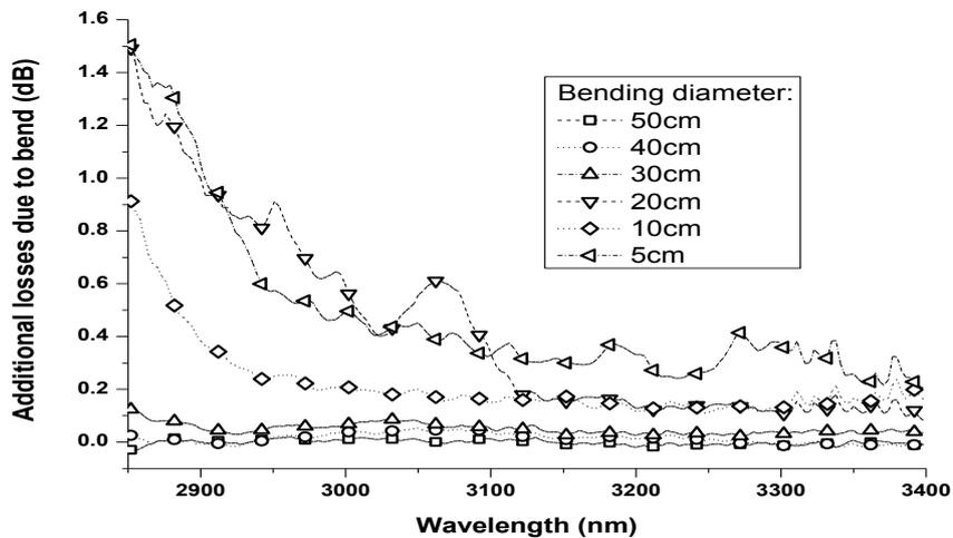
Figure 5: Additional losses due to a 180° bend in a 1.23 m long NCF.
