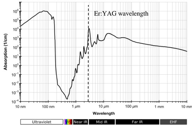
**Figure 1: Absorption of water versus wavelength from [2]**
