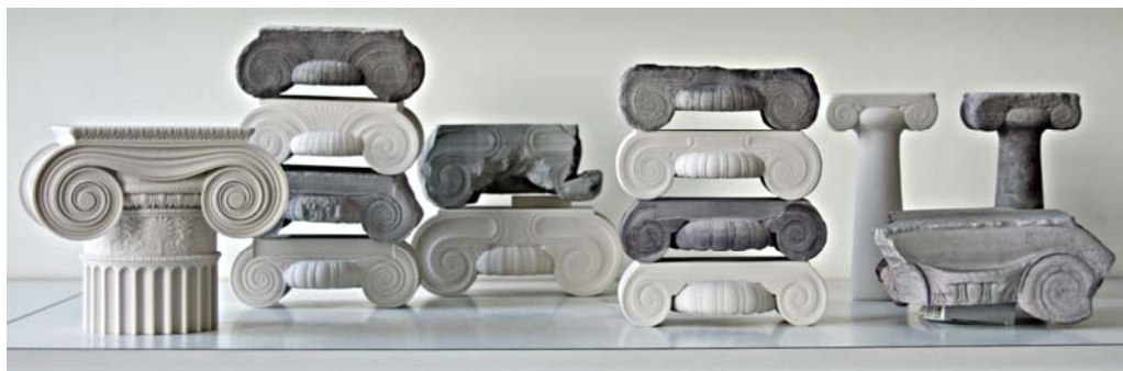
Figure 7. Facsimiles made by 3D printing from laserscans (dark) and restored Rhino models (light). In the centre are various Cycladic forms; on the left is the canonical Ionian version from the Erechtheion.
