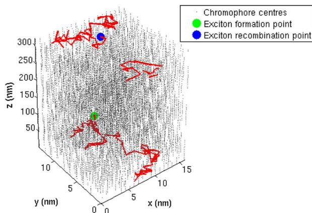
**Fig. 5.** Trajectory of an exciton created at the point (5, 10, 100) that recombines at the point (10, 10, 300) on an ordered chain morphology. Note that periodic boundary conditions have been used. (Taken from [14].)
