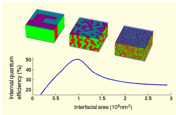
**Fig. 8.** Internal quantum efficiency (%) versus interfacial area ( $10^6 \text{ nm}^2$ ) and example morphologies generated by minimization of an Ising Hamiltonian. Electron and hole conductors are displayed as dark (red in color plot) regions and light (green in color plot) regions, respectively. The anode and cathode (blue in color plot) are the top and bottom planes and are separated by 90 nm. (Table of contents plot from [41].)
