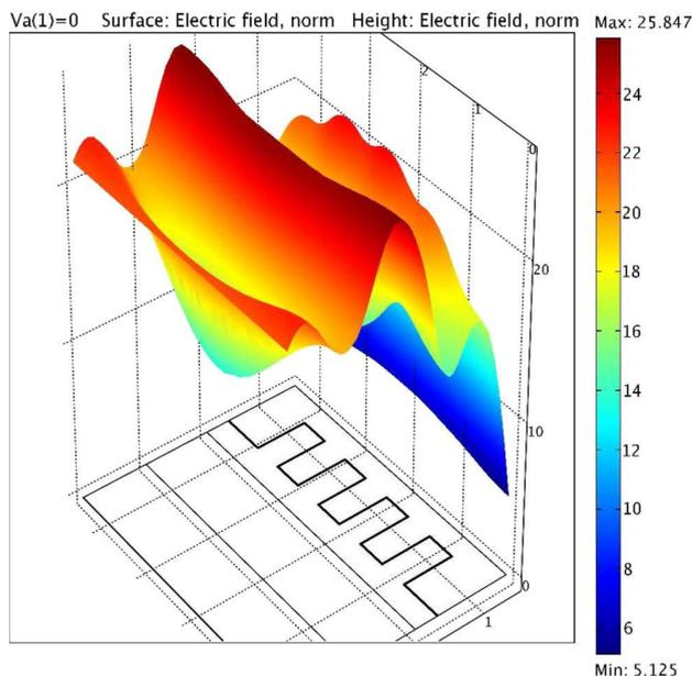
**Fig. 9.** Example plot of the magnitude of the optical electric field (in  $\text{Vm}^{-1}$ , with values from 5.125 to 25.847  $\text{Vm}^{-1}$ ) inside a device at 0.1 Sun. The figure also shows the underlying device morphology. (Taken from [46].)
