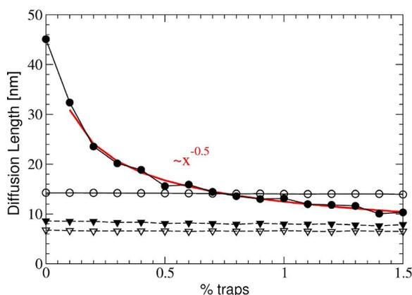
**Fig. 7.**  $L_D$  variation with the percentage of sites occupied by traps  $x$ . Solid lines:  $T = 294$  K; dashed lines  $T = 7$  K. Filled circles indicate intra- and interchain hops permitted; empty circles are for intra-chain hops only. The line showing  $L_D$  varies as  $x^{-0.5}$  comes from the prediction of [35]. (Taken from [14].)
