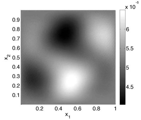
FIG. 8. Simulation using the same parameters as in Fig. 7 but employing the polynomial energy landscape from Ref. 3. Shown is the order parameter  $\varrho_0$ , as in the bottom panel of Fig. 7. No clear distinction between the phases can be observed (note that the scaling of the order parameter is  $10^{-5}$ , so the variation is 2 orders of magnitude smaller).
