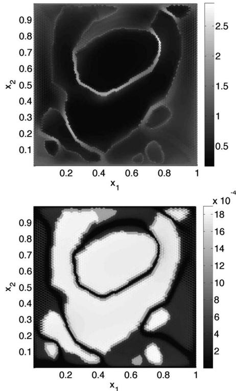
FIG. 9. Elastic energy density (top panel) and order parameter  $\varrho_0$  (bottom panel) of the fully relaxed state of a simulation with initial and boundary conditions on a rank-1 connection in between the tetragonal and the monoclinic minima of the energy. A complex arrangement of phases has formed, with boundaries of higher energy in between.
