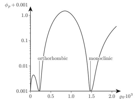
FIG. 6. The profile  $\phi_p$  along the path from the tetragonal phase (left, at the origin) via the orthorhombic phase (middle) to the monoclinic phase (right). Since the path is a function of  $\varrho_0 = (e_1 - e_2)^2$ , only non-negative arguments are meaningful.
