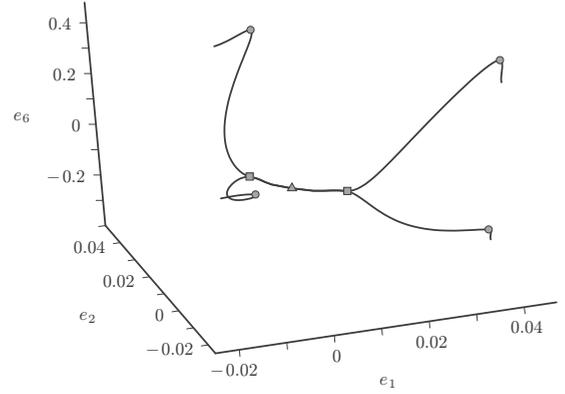
FIG. 5. Diagram of the paths in strain space (the image of these paths under  $\varrho$  is the path shown in Fig. 4). The paths emerge at the tetragonal phase (triangle) in the origin and remain in the  $e_1$ - $e_2$  plane before bifurcating at the orthorhombic phases (square) in order to reach the monoclinic phases (circle).
