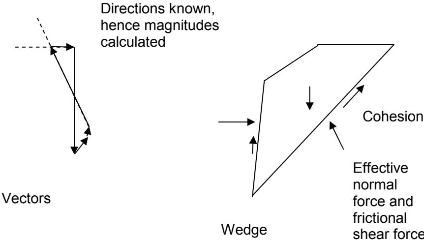
Figure 4 Determination of forces on first wedge
