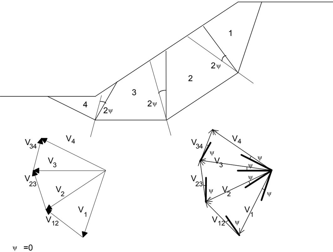
Figure 2 Hodograph for a four wedge mechanism. The thick lines in the hodograph on the right are the orientations of the surfaces.
