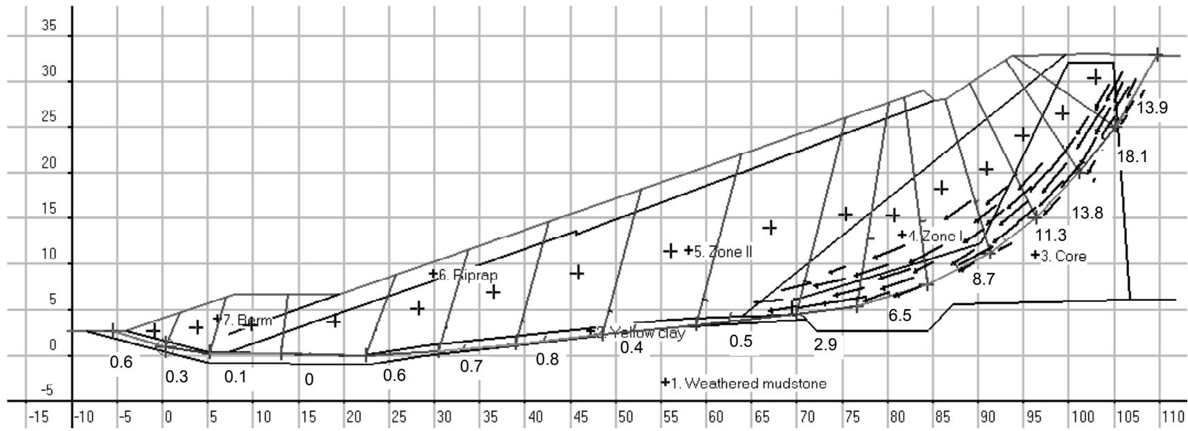
Figure 6 Analysis of Carsington embankment from the computer screen, with vectors from finite element analysis [Potts et al.] added to show shape of failure surface through the core and the 'boot'. The numbers beneath the slip surface indicate the displacement beyond peak, as a percentage of the displacement to peak strength.
