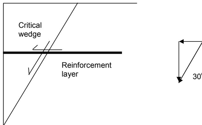
Figure 7 Strains in reinforcement in a vertical reinforced soil wall
