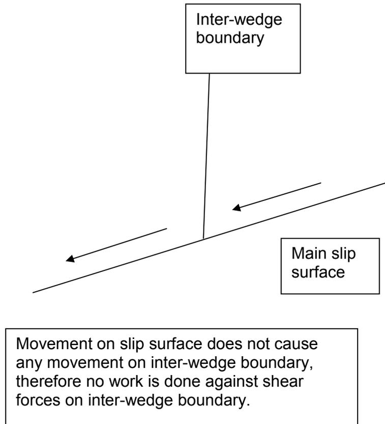
Figure 1 Relative displacement between wedges
