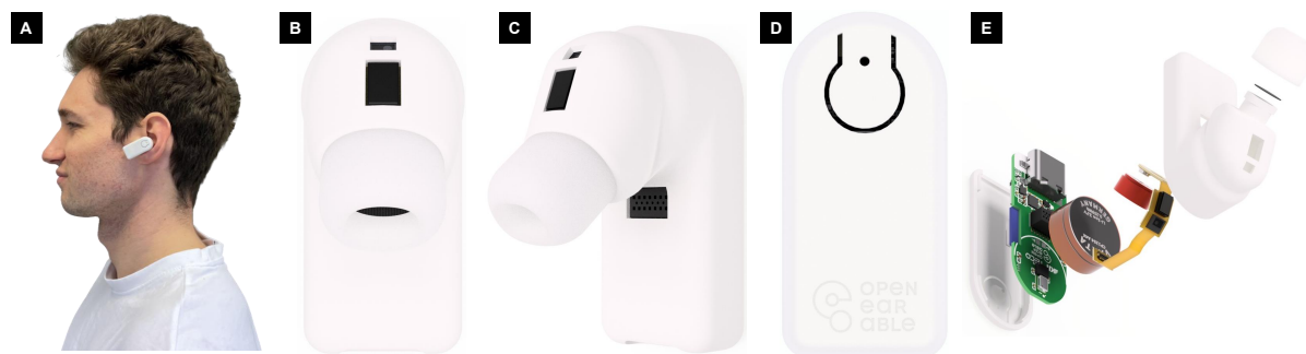
Fig. 1. (A) a user wearing OpenEarable 2.0; (B) the front view of the device revealing a pulse oximeter and optical temperature sensor; (C) the frontal-right view of the device showing its shape and extension connector; (D) the back view of the device showing the push button and microphone hole; (E) an explosion rendering of OpenEarable 2.0, revealing three microphones (inside the ear canal, external facing, and bone-conduction), a pressure sensor, a 9-axis IMU for measuring head movements, a 3-axis accelerometer for measuring movement in the ear canal, a coin cell battery, a speaker and a dual-core LE Audio capable microcontroller.
