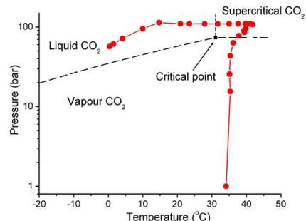
Fig. 1. (Color online) Measured supercritical drying cycle on a CO<sub>2</sub> phase diagram. The pressure and temperature were recorded every 5 min and marked by dots. The liquid-vapor phase boundary is not crossed; the liquid and vapor phases are never present at the same time.
