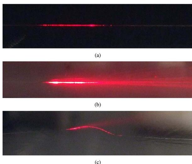
Fig. 3. (Color online) Photos of embedded tapered fibers with waist diameters of (a)  $10\ \mu\text{m}$ , (b)  $2\ \mu\text{m}$ , and (c)  $1\ \mu\text{m}$ . The fibers carry red laser light from left to right. Noticeable scattering begins at the start of the 1-cm-long waist. The paths of the scattered light through the aerogel can be seen. The images are  $\sim 3.1\ \text{cm}$  long.
