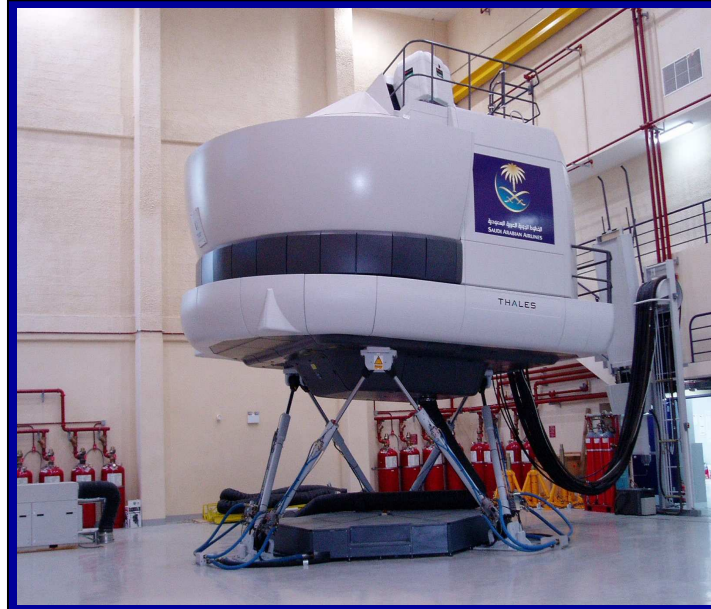
Fig. 1 Full flight training simulator
