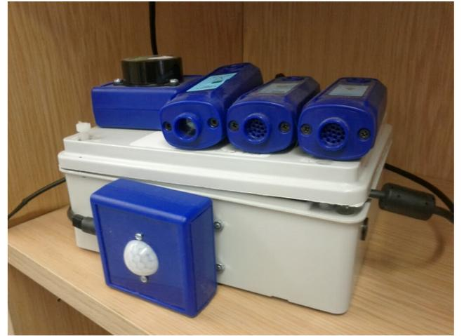
**Figure 1: Sensor box *in situ.*, showing PIR, temperature, CO<sub>2</sub>, light, sound and humidity sensors.**
