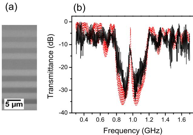
FIG. 4. (Color online) (a) SEM image of acoustic microcavity structure (thickness of  $\sim 20 \mu\text{m}$ ). (b) Acoustic longitudinal wave transmission through pSi microcavity structure. Solid curve: measured transmittance spectrum normalized as in Fig. 1. Dashed curve: calculated transmittance.
