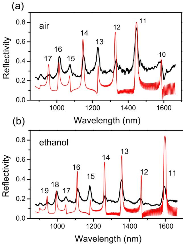
FIG. 2. (Color online) Thick curves: optical reflectivity spectra measured for DBR with pores filled by (a) air and (b) ethanol. Thin curves: the results of fitting procedure using parameters  $n_i$  and  $d_i$  indicated in the text. Numbers indicate the order  $m$  of the optical stop bands.
