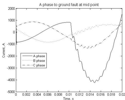
Figure 8: Current waveforms for an A-phase-earth fault
