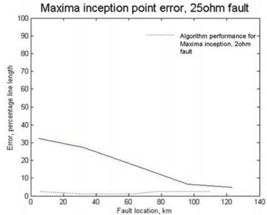
Figure 11: Response for fault resistance of 25 ohms
