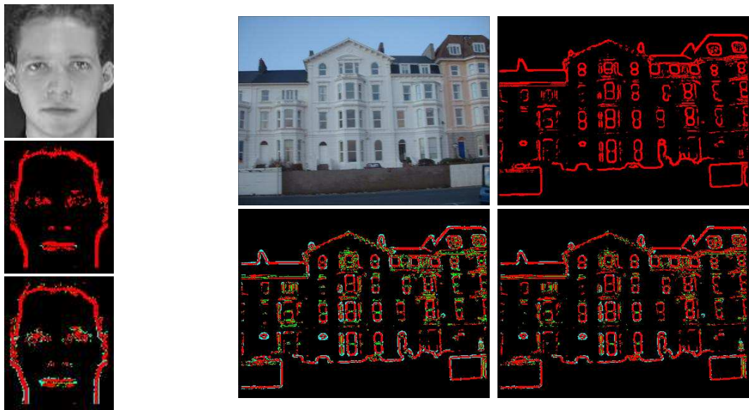
Figure 5: Incremental learning applied to low-level feature classification using an additive GMM classifier. Features to be classified are “edge” (red) “ridge” (green), “corner” (cyan), or “none” (black). Left column, from top: face picture; “face” classifier only; combined classifier. Right columns, top-right to bottom-left: houses picture; houses with “face” classifier; houses with “house” classifier only; combined classifier result.
