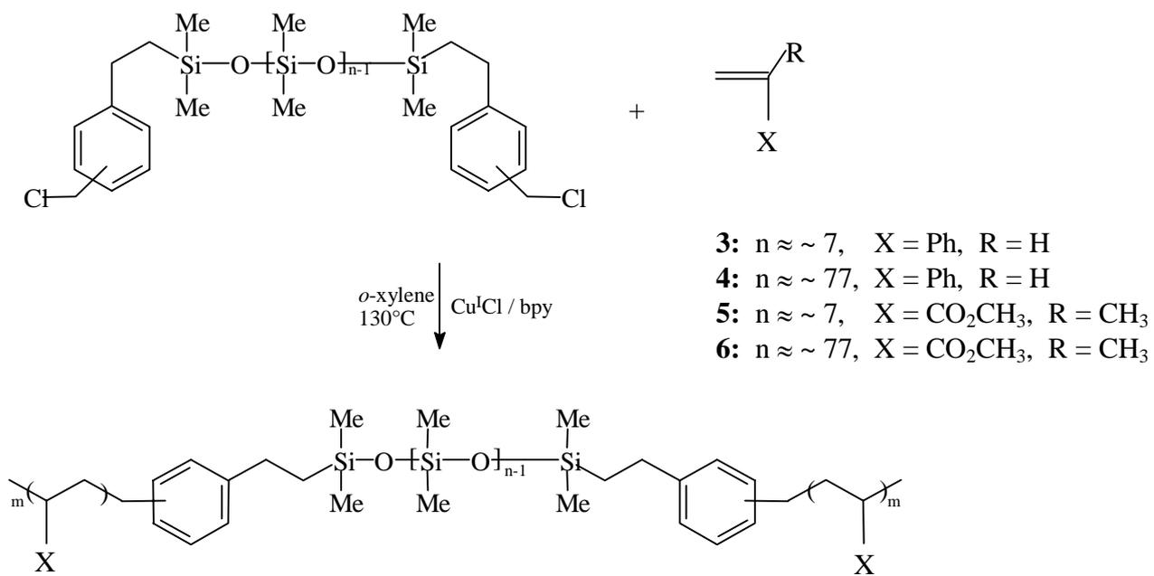
**Scheme 2.** ATRP synthesis of PDMS block copolymers
