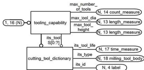
Fig. 5. The EXPRESS-G diagram of cutting\_tool\_dictionary.
