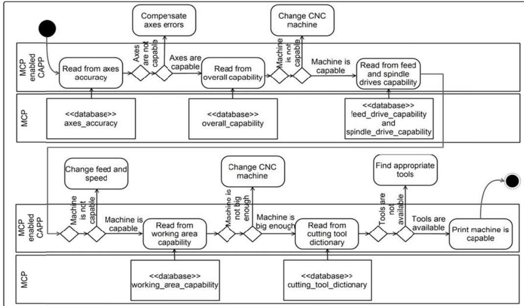
Fig. 2. UML activity diagram of manufacturing capability tests.
