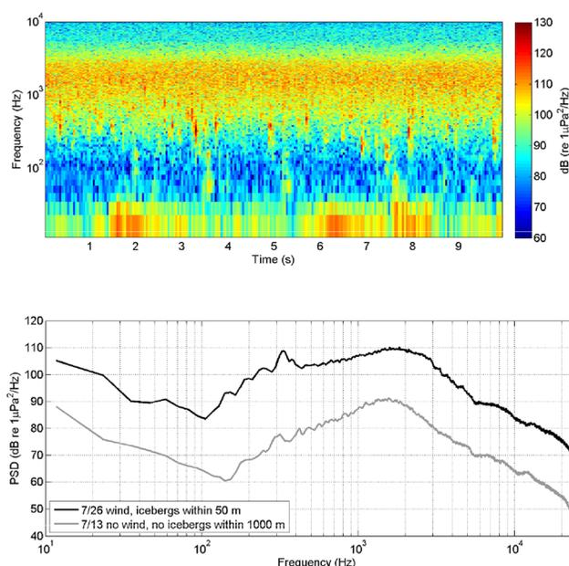
FIG. 3. (Color online) Top: A spectrogram of 10 s of ambient noise measured at site 130726/1 (see Fig. 1). Bottom: Noise power spectral density averaged across the 10 s recording interval.
