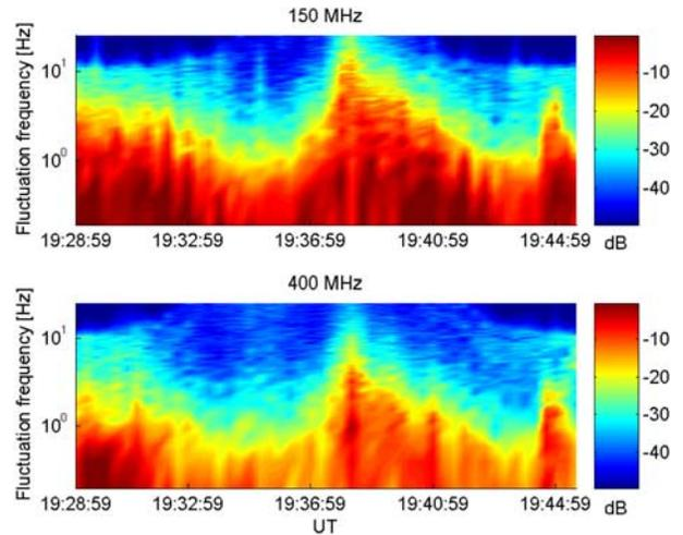
**Figure 4.** Overview of the intensity spectra observed at 150 MHz and 400 MHz at the ground station located in Kokkola during the night of 30 October 2003, for a satellite pass starting at 19:28:59 UT.
