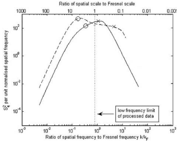
**Figure 9.** Theoretical intensity spectra calculated on the basis of the refractive theory for the observed spectra shown in Figure 8. Also, the lens scale ('o') and the focal scale ('x') are shown. The vertical dotted line represents the low frequency limit of the detrended experimental data.
