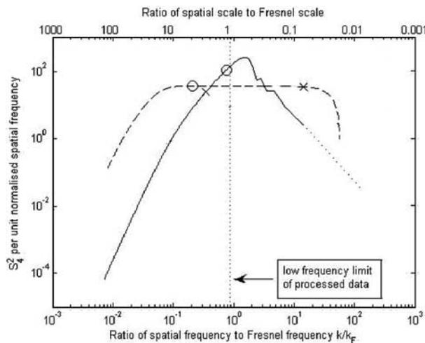
**Figure 7.** Theoretical intensity spectra calculated on the basis of the refractive theory for the observed spectra shown in Figure 6. Also, the lens scale ('o') and the focal scale ('x') are shown. The vertical dotted line represents the low frequency limit of the detrended experimental data.
