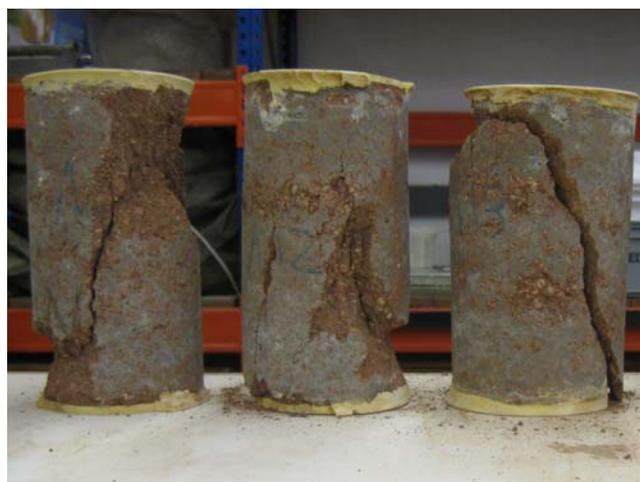
Figure 7. Tested triaxial specimens
