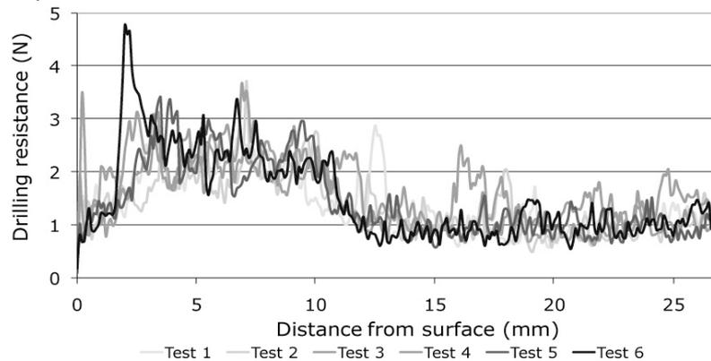
Figure 1: Raw DRMS data for 90 day-old lime mortar
