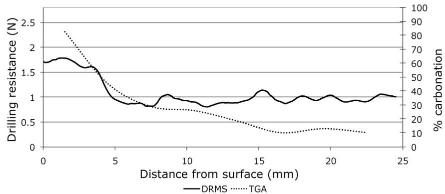
Figure 5: TGA carbonation data superimposed on adjusted DRMS data at 28 days.
