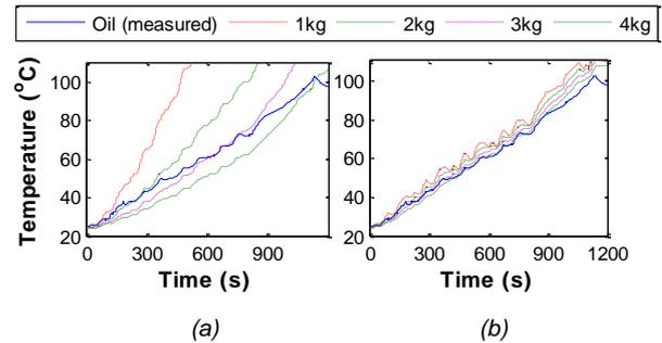
Figure 16: Coolant temperature for (a) *heat-to-coolant* and (b) *heat-to-coolant-to-oil* simulations for different thermal inertias of the additional heat exchanger system (thermal inertia expressed as equivalent water mass)
