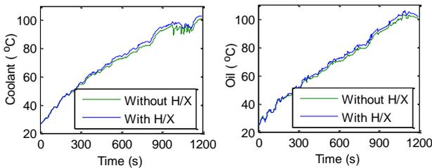
Figure 10: Coolant and oil temperatures with and without heat exchanger heat exchanger hardware installed
