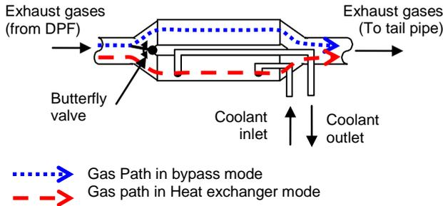
Figure 2: Exhaust gas heat exchanger layout and operation
