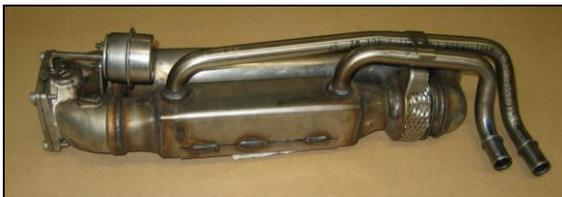
Figure 3: Exhaust gas heat exchanger
