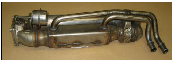
Figure 3: Exhaust gas heat exchanger
