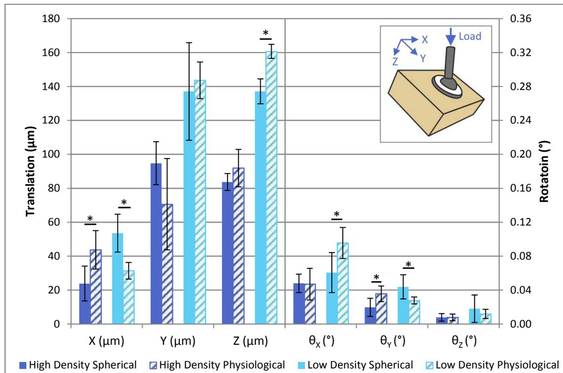
**Figure 4.** Comparing the micromotion of the acetabular cup in six degrees of freedom when implanted in Spherical and Physiological (0.08° corresponds to 40  $\mu\text{m}$  with this specific implant). Values expressed as mean and standard deviation. \* Statistically significant difference ( $P = 0.05$ ) with Mann-Whitney test.
