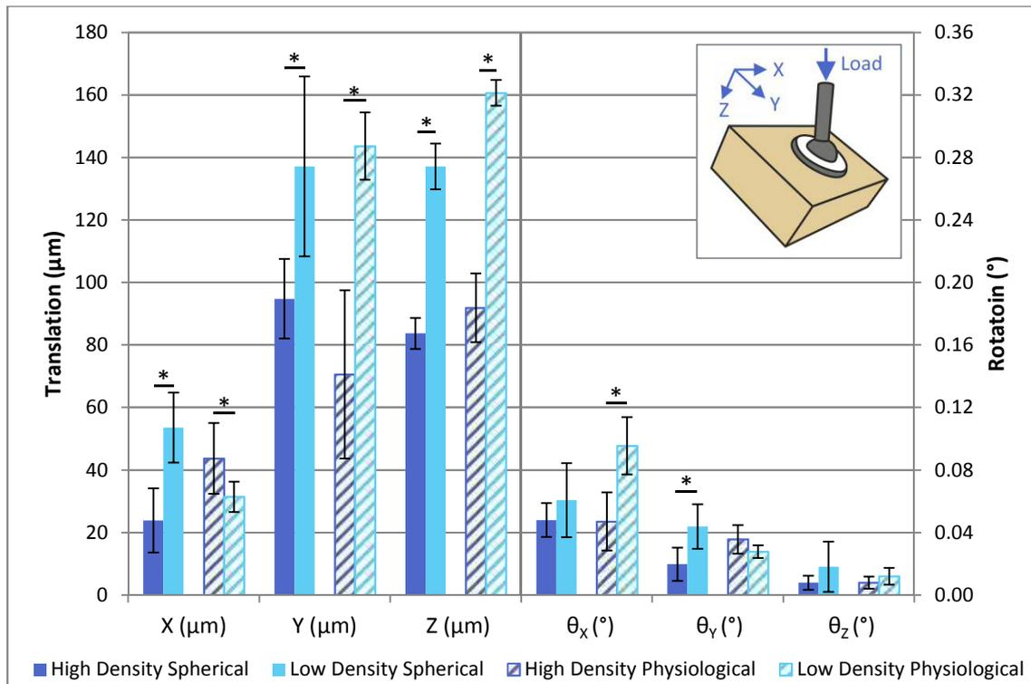
**Figure 6.** Comparing the micromotion of the acetabular cup in six degrees of freedom when implanted in High and Low Density foam blocks (0.08° corresponds to 40 µm with this specific implant). Values expressed as mean and standard deviation. \* Statistically significant difference ( $P = 0.05$ ) with Mann-Whitney test.
